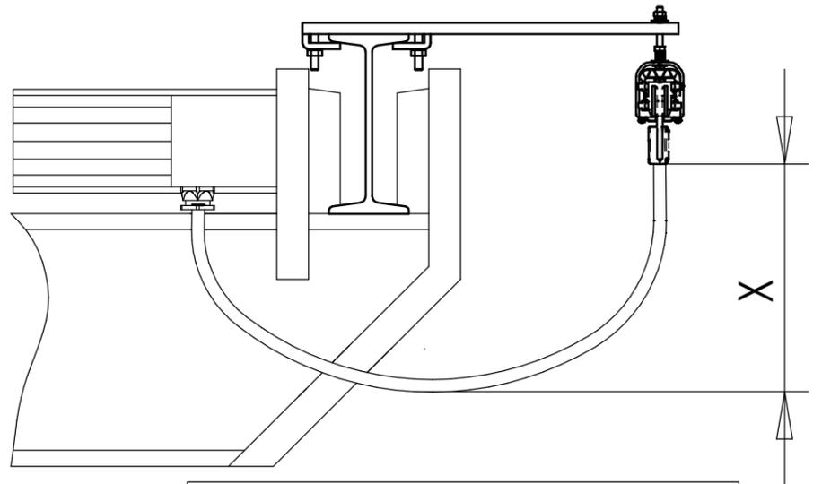
**Cable / Cable / Kabel / Cable H07 RNF**
